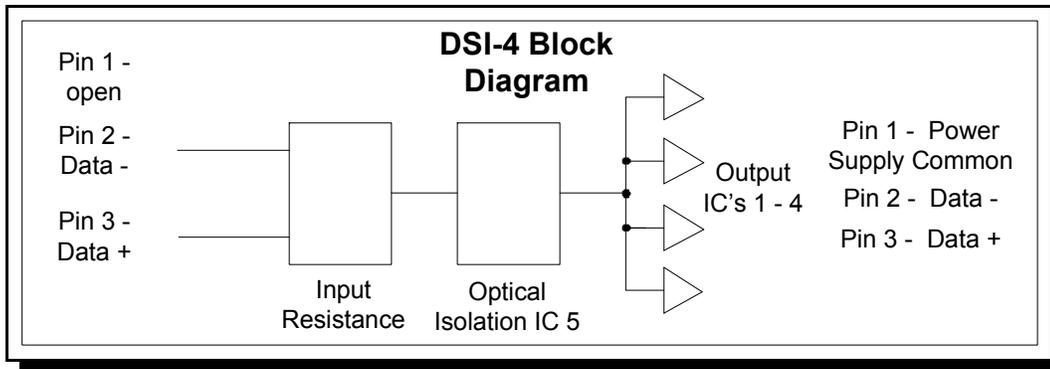
**INPUT:** The input stage has a 68 ohm resistor in series with pin 2 and a 68 ohm resistor in series with pin 3 connecting to the input of IC #5 (*Optically isolated input IC*). There is a 2.2K ohm resistor and the front panel LED (*data indicator LED*) in parallel to the input of IC 5.
