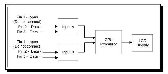
**INPUT:** The inputs (pins 2 and 3) connect to a 75176 data input IC's, and send to the processor.
