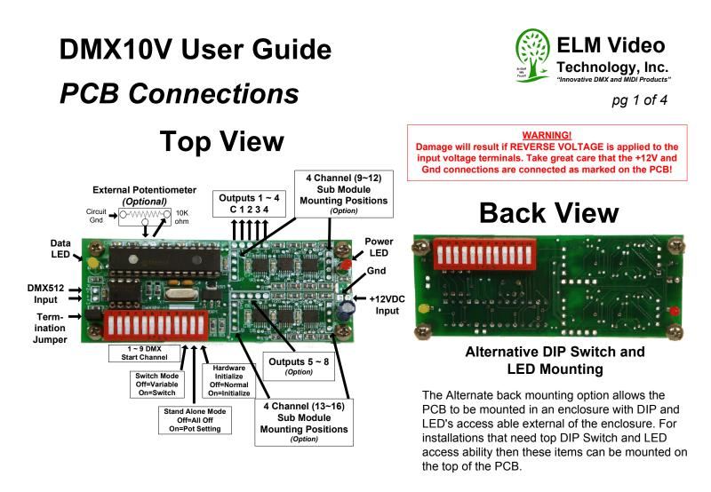
To install the LED's and DIP switch, decide which side (front or back) of the PCB to mount the components back. If the PCB will be mounted inside an enclosure that only needs access internally then mount the components on the top. If the installation requires seeing the LED's and access to the DIP switch's are needed then mount the components on the back. Once the holes are made in the enclosure mount the PCB and wire as shown in the "DMX10V Drill Template and Wiring Diagram" Document.
