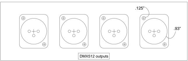
Dimensions for Neutrik 3 or 5 Pin Male/Female Chassis Mount XLR's. Any 3 or 5 pin XLR type can be used; chassis mount or inline.
